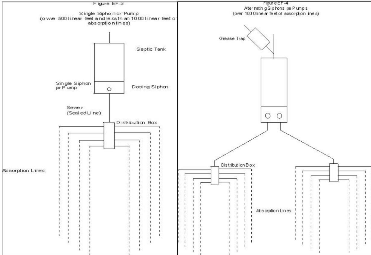
g. Design and Operation of Dosing Tank with Pump(s).
