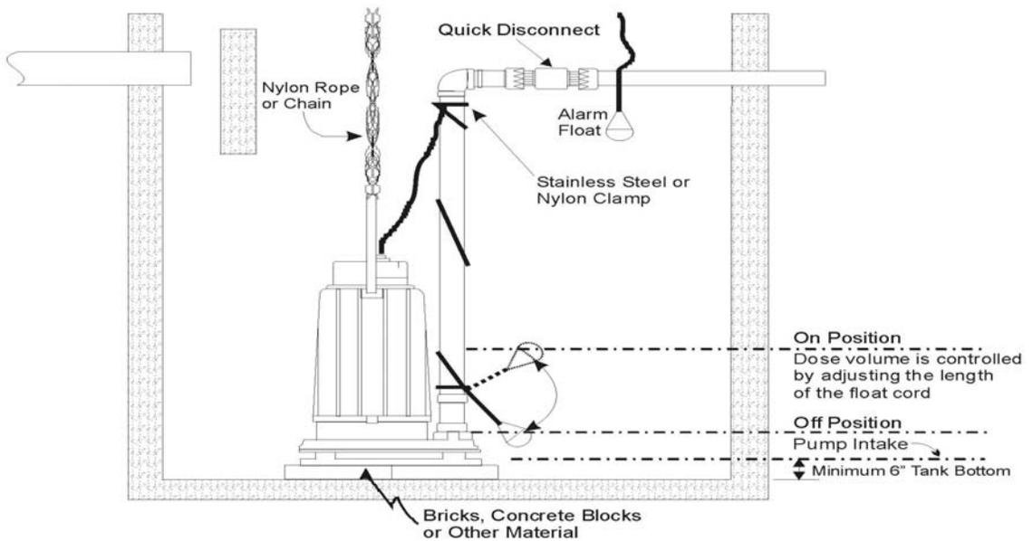
NOTE: Sufficient horizontal distance must be provided for the float to move freely.
