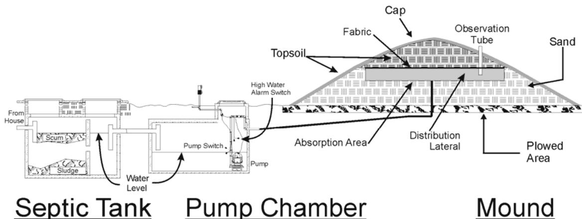
Figure 1. Cross-section of a Wisconsin mound system
