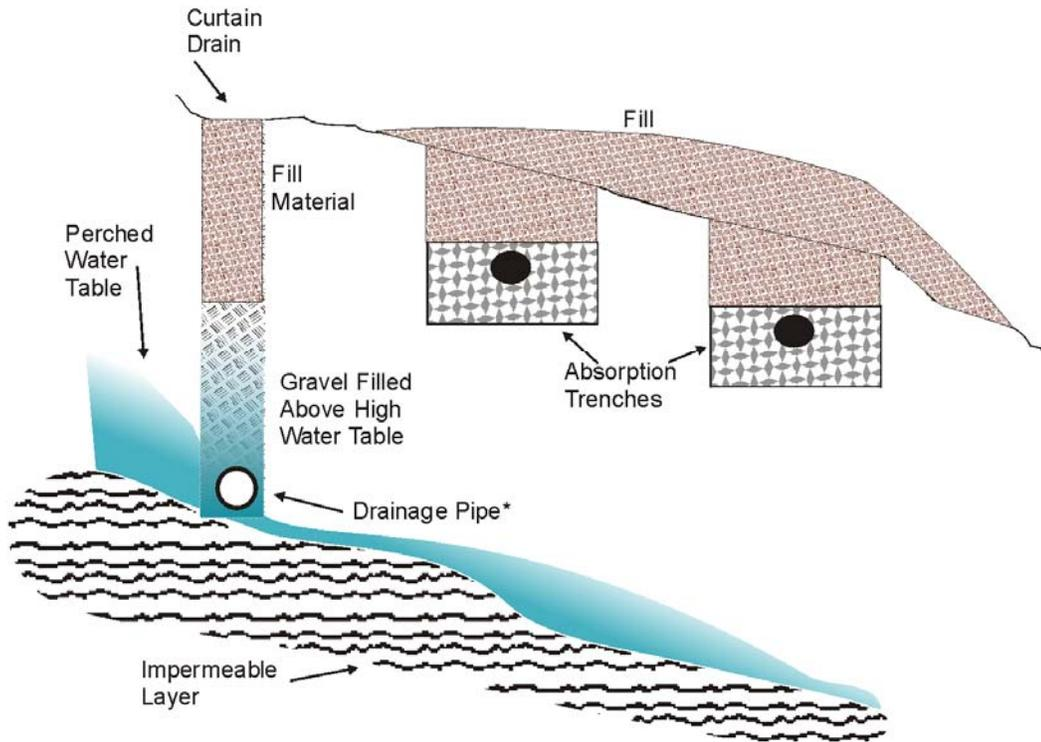
\*Joints or perforations should be covered by treated building paper or pipes jacketed with mesh
