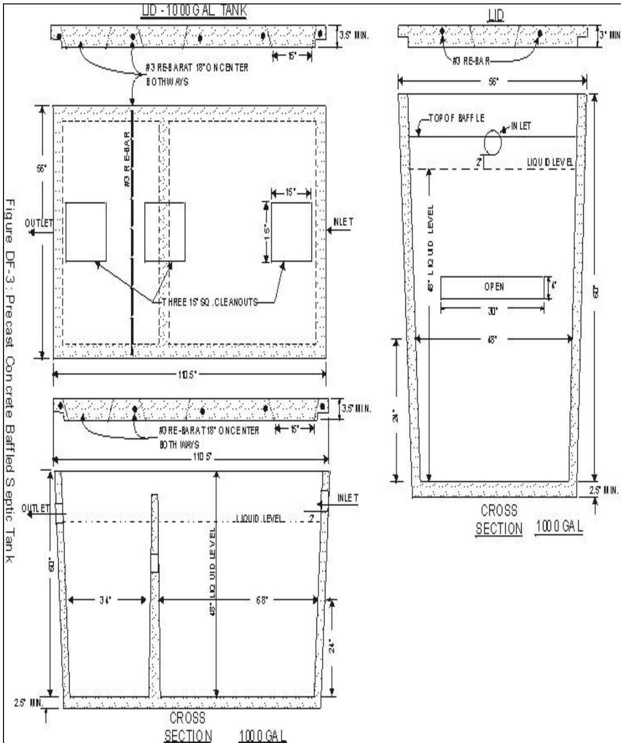
Figure DF-3: Precast Concrete Baffled Septic Tank
