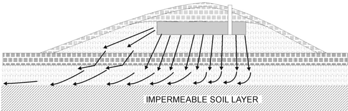
Figure FF-13 Effluent Movement Within and Away from the Wisconsin Mound for Four Different Types of Soil Profiles
