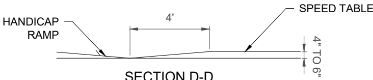
SECTION D-D TYPE 2 SPEED TABLE DETAIL NTS
