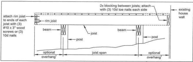
FIGURE 4: JOIST SPAN - FREE-STANDING DECK2
