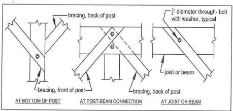
FIGURE 24: TYPICAL CONNECTIONS OF DIAGONAL MEMBERS
