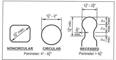
FIGURE 37: HANDRAIL GRASPABILITY TYPES/GEOMETRY
