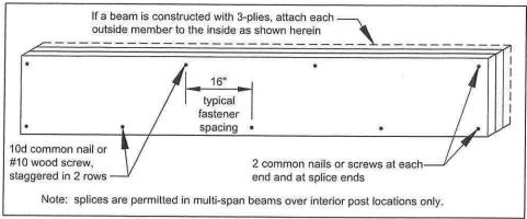
FIGURE 6: BEAM ASSEMBLY DETAIL
