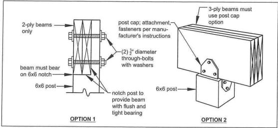
FIGURE 11: POST-TO-BEAM CONNECTION OPTIONS
