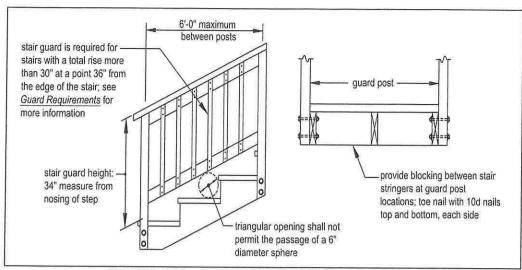
FIGURE 36: STAIR GUARD REQUIREMENTS
