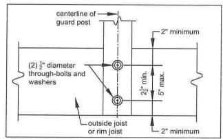
FIGURE 29: GUARD POST ATTACHMENT DETAIL
