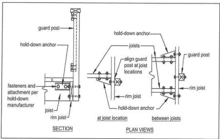
FIGURE 31: GUARD POST-TO-RIM JOIST DETAIL
