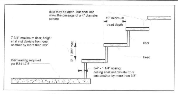
FIGURE 32: TREAD AND RISER DETAIL
