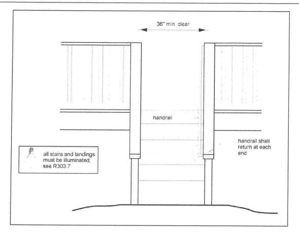
FIGURE 39: MISCELLANEOUS STAIR REQUIREMENTS
