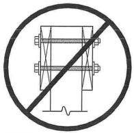
FIGURE 10: PROHIBITED POST-TO-BEAM ATTACHMENT
