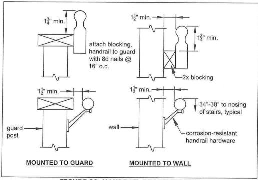
FIGURE 38: HANDRAIL REQUIREMENTS
