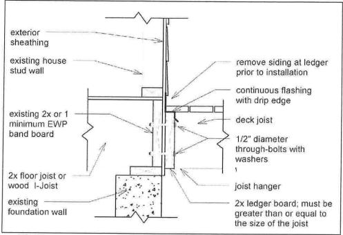
FIGURE 14: ATTACHMENT OF LEDGER BOARD-TO-BAND BOARD
