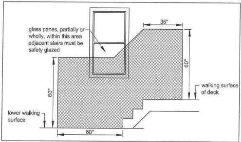
FIGURE 42: SAFETY GLAZING AREA AT STAIRS
