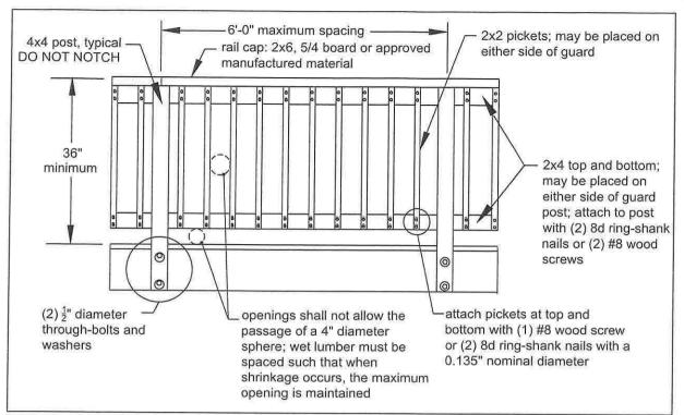
FIGURE 27: TYPICAL GUARD DETAIL
