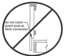
FIGURE 28: NOTCHING AT GUARD POSTS
