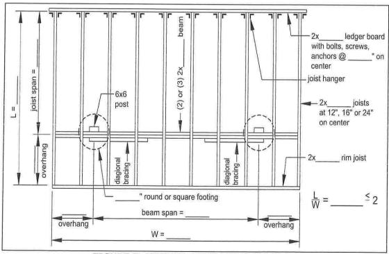
FIGURE 7: TYPICAL DECK FRAMING PLAN
