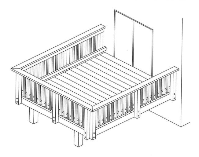
This design document applies to <u>single-span</u>, <u>single-level</u> <u>residential</u> decks only. Decks must be constructed in conformance with the details contained herein. A copy of this deck detail must be on the job site and available to the inspector during each required inspection.
