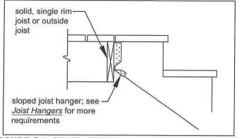
FIGURE 34: STAIR STRINGER ATTACHMENT DETAIL
