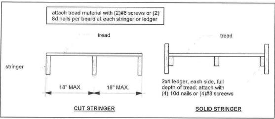
FIGURE 35: TREAD CONNECTION REQUIREMENTS
